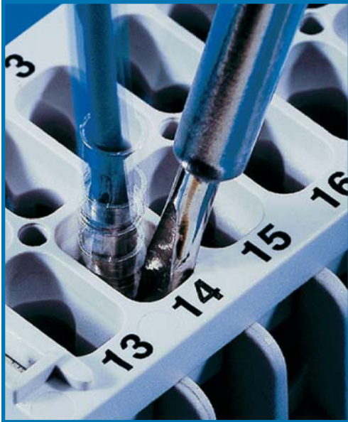
Use small blade screwdriver to push wire entry tab in for easy contact removal
